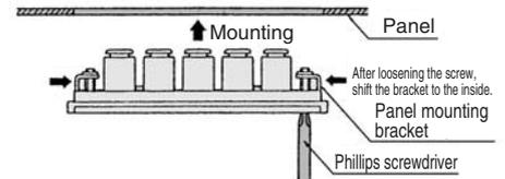
3. After shifting the bolt for bracket to the outside, tighten the bolt by a Phillips screwdriver to fix the socket case.
