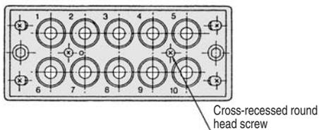
2. After exchanging connectors in desired places, fix the plate to the case by using a Phillips screwdriver.
